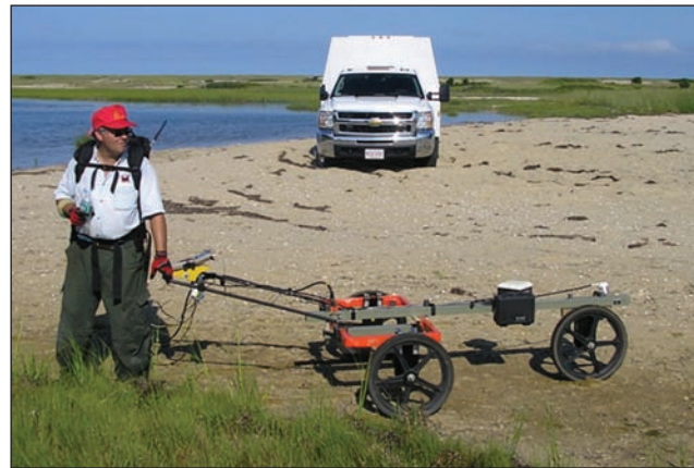
Bob Selfridge uses a man portable simultaneous electromagnetic and magnetic detector to look for potential buried munitions at Martha's Vineyard, Mass.
