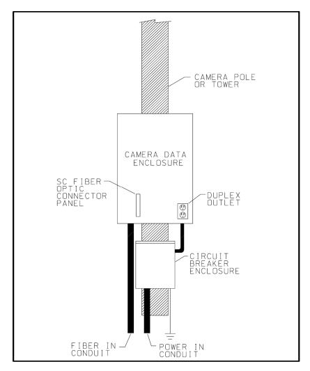
Example Exterior Camera Enclosure (Not to Scale)
