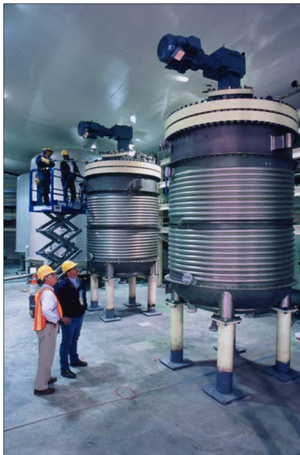
Figure 3.5 Officials inspect the neutralization reactors at Aberdeen prior to operations startup in 2003 (CMA photo).
