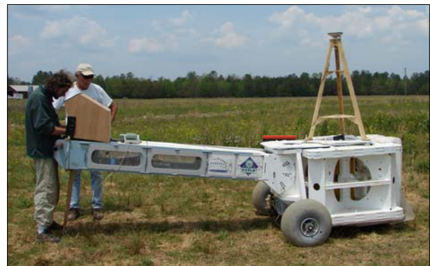
Figure 4.3 Berkley UXO Discriminator, one of several prototype discrimination tools tested at Camp Sibert.
