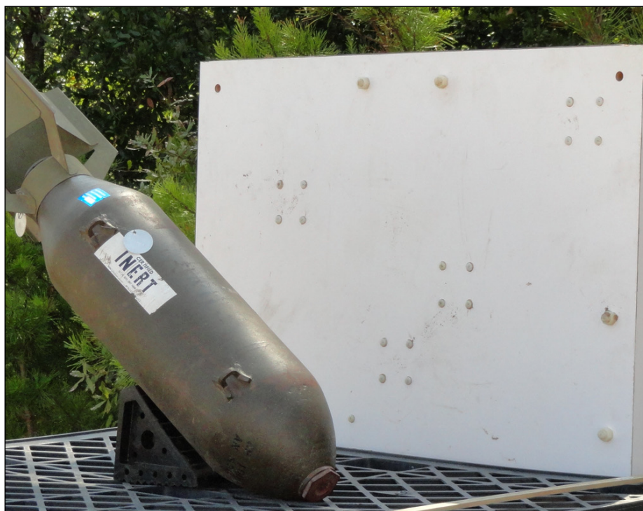
In Florida, one of the munitions the MetalMapper used to collect advanced electromagnetic induction signatures was the inert, 100-pound general purpose practice bomb provided by Navy and Air Force museums in the area there.
