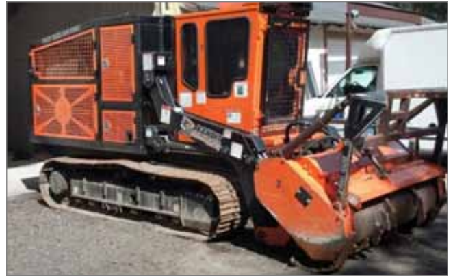
A mulcher used in vegetation clearance on Army ranges
