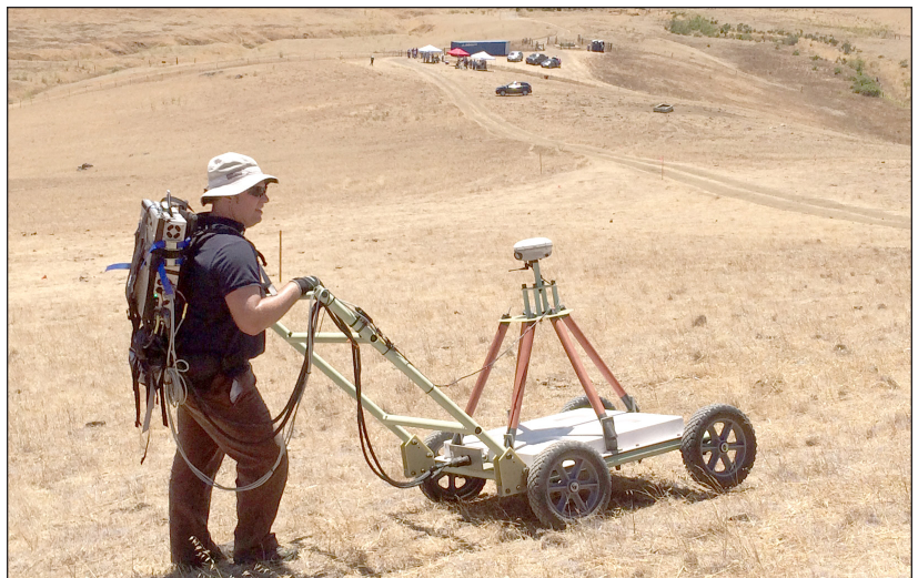
A technician uses a TEMPTADS sensor platform for a technology demonstration at the Formerly Used Defense Site (FUDS), Camp San Luis Obispo, California.
