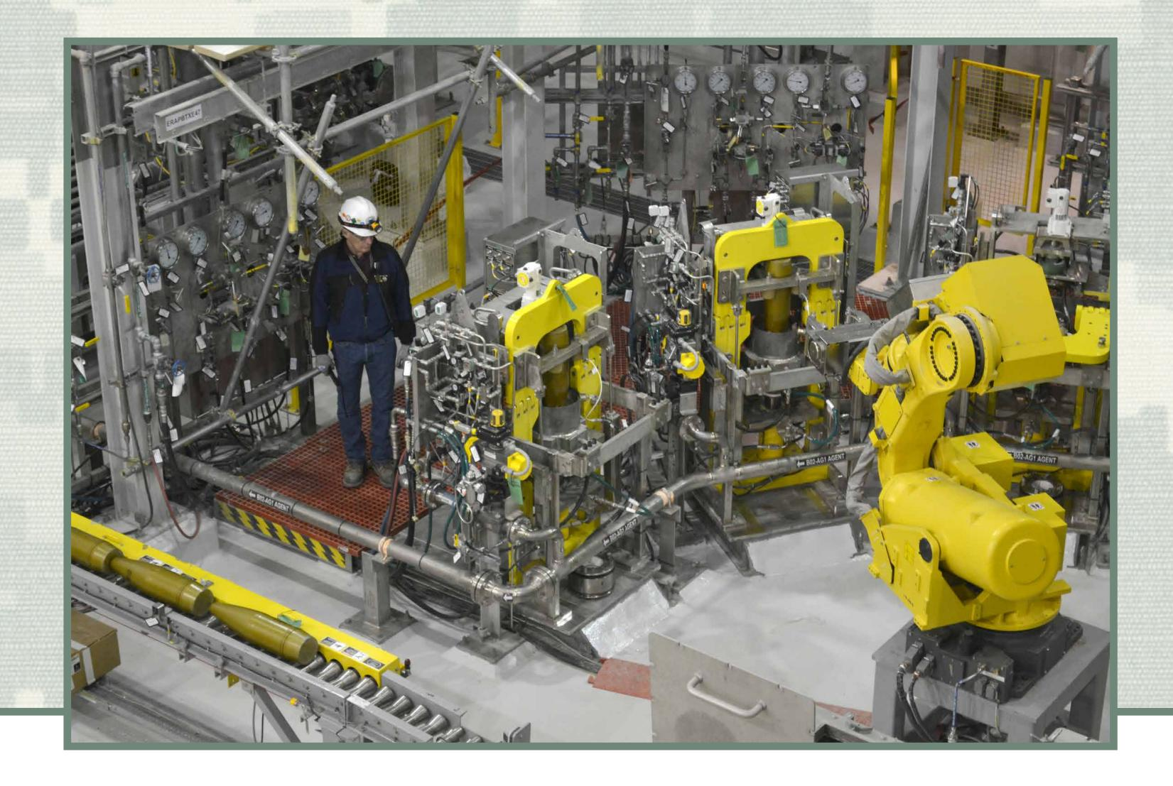
For each disposal site, Huntsville Center staff has developed initial facility design requirements and identified appropriate equipment based on the approved destruction technology. Inside the Agent Processing Building of the Pueblo Chemical Agent Destruction Pilot Plant, a start-up specialist tests the Cavity Access Machines of the Munitions Washout System. Specialized robots, also procured by Huntsville Center, transfer materials to the appropriate stations.
